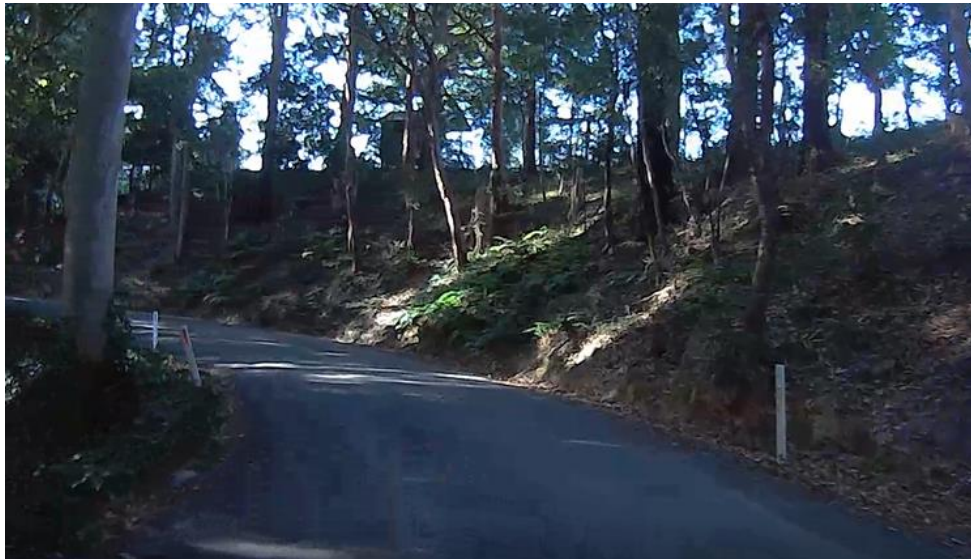
Photo 4: Example 2 of narrow shoulders/inadequate roadside drainage
